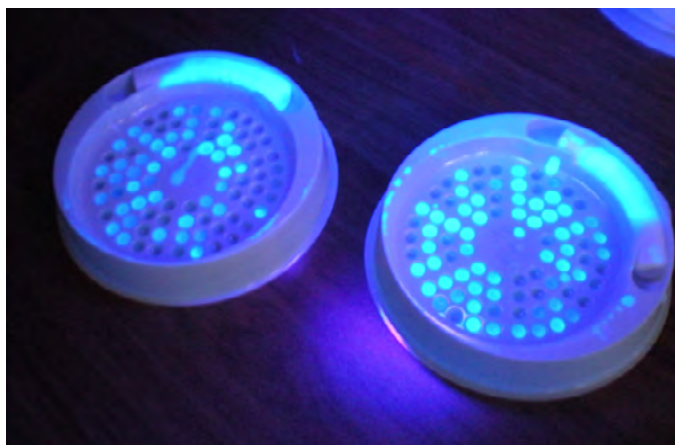
FIGURE 5. SimPlates under UV light, for measuring Total Cultivable bacteria (TCB)
