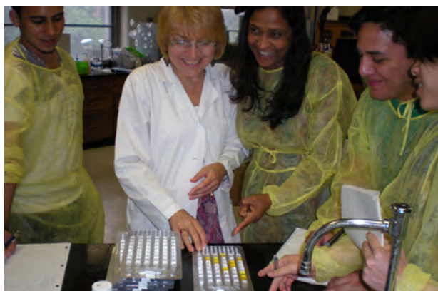
FIGURE 6. QuantiTray with large and small wells for measuring the number of coliforms; In the Microbiology Lab with Prof. Tsenova and Prof. Ghosh-Dastidar
